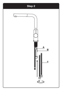
Connect the hot and cold flexible hoses (C) to the inlets (A & B) on the bottom of the tap by twisting them clockwise until tight and secure.
