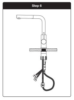
Connect the hot and cold supply hoses to the isolating stop valves beneath the sink and tighten until secure.
