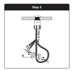
Undo the counterweight (K) and place around the pull-out hose in a position that allows the showerhead to retract all the way back in when pulled out.
