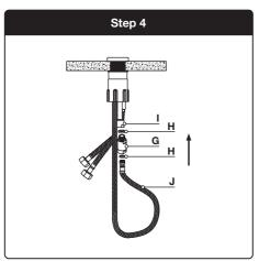
Insert a rubber washer (H) into the inlet pipe
