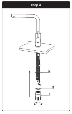
**3.** Insert the tap into a 35mm hole in the sink or benchtop.
