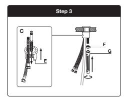
3. Insert the tap into a 35mm hole in the sink or benchtop and secure underneath by sliding the tap brace (E) onto the mounting bolt (C).
