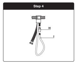
Screw the non-return valve (H) onto the mounting bolt and tighten. On the other end of the non-return valve, check that the pull-out hose (I) is secure and tight.
