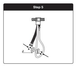
Undo the counterweight (J) and place around the pull-out hose in a position that allows the showerhead to retract all the way back in when pulled out.
