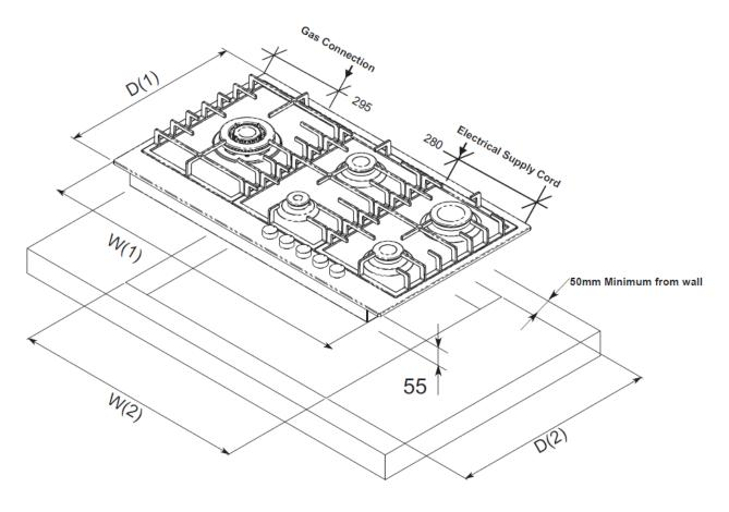
Product dimensions 55mm (H1), 890mm (W1), 510mm (D1) Cut out dimensions 805mm (W2), 480mm (D2)
