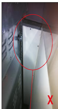
Left Side of oven, chain not attached
